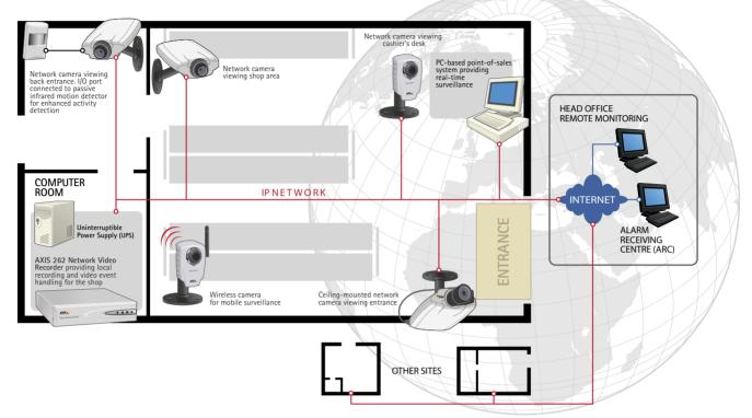
In an Axis network video solution, the cameras are connected directly to your IP network, eliminating numerous coaxial cable runs. Video streams delivered by local or remote network cameras are recorded at pre-defined rates according to a specific schedule or upon detection of motion. Live video and recorded archives are viewable from any authorised PC connected to the local network or the Internet.
