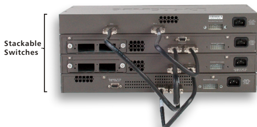
xStack™ - Ring (Bus) Architecture
