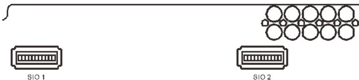
Figure 3- 5. SIO 1 and SIO 2 Stacking ports at the rear of the DGS-3324SR
